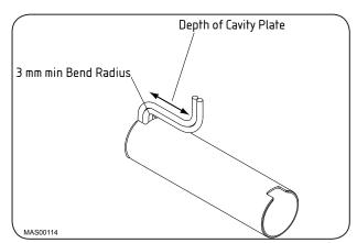
2. Bend the heater wires as shown above.
