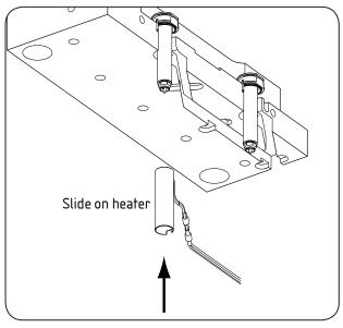
5. Slide the heaters on to the nozzles and thread the wires through the wire channel.
