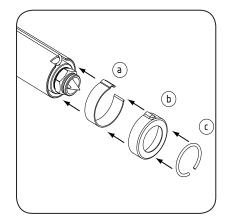
Install the T/C clip (a), the heater cap (b), and snap ring (c) (in that order).
