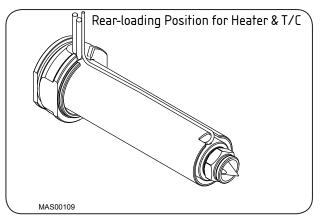
Bend the T/C along the outside of the heater and bend it again with the heater wires at the nozzle head.
