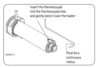
Insert the T/C in the hole near the nozzle tip and bend it over the heater as shown.
