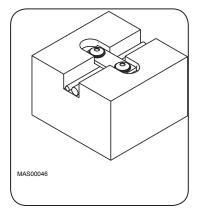
Attach the wire clips over the wires in the wire channels.
