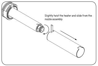
Slightly twist the heater and slide it off the nozzle. Take care not to break the heater wires.
