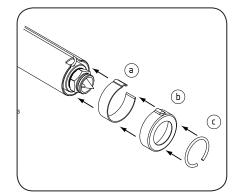
8. Install the T/C clip (a), the heater cap (b), and the snap ring (c) (in that order).
