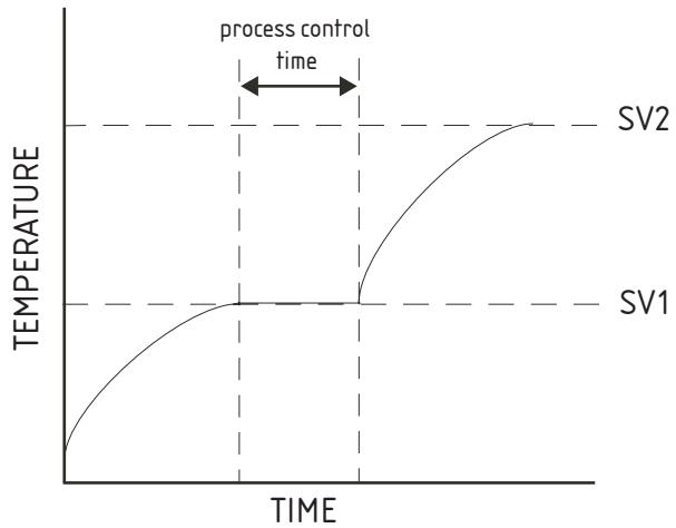
On start up the temperature will increase to the set SV1 parameter. It will remain at this temperature for the set process control time (PCT). The temperature will then increase to the set SV2 parameter.
